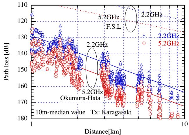
Fig. 12 Path loss vs. distance in Karagasaki-Chofu measurement
