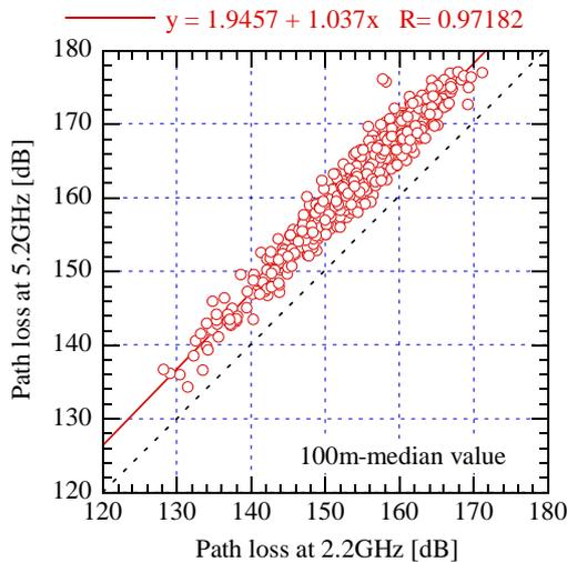
Fig. 4 Path loss correlation between 2.2 GHz and 5.2 GHz in Shinjuku-Kawagoe measurement obtained from 100-m median value
