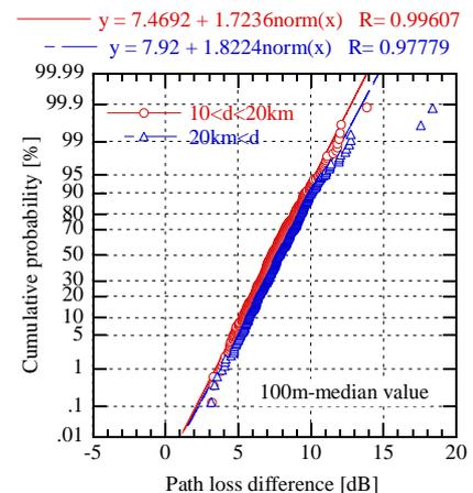
Fig. 8 Cumulative probabilities of the difference in path loss between 2.2 GHz and 5.2 GHz in case of 100-m median value
