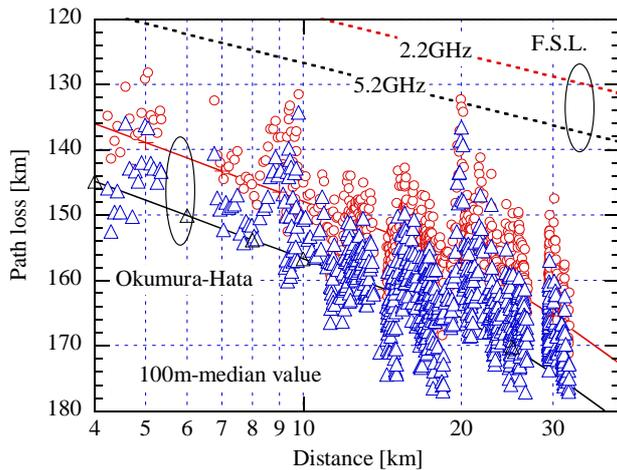
Fig. 2 Path loss vs. distance in Shinjuku-Kawagoe measurement
