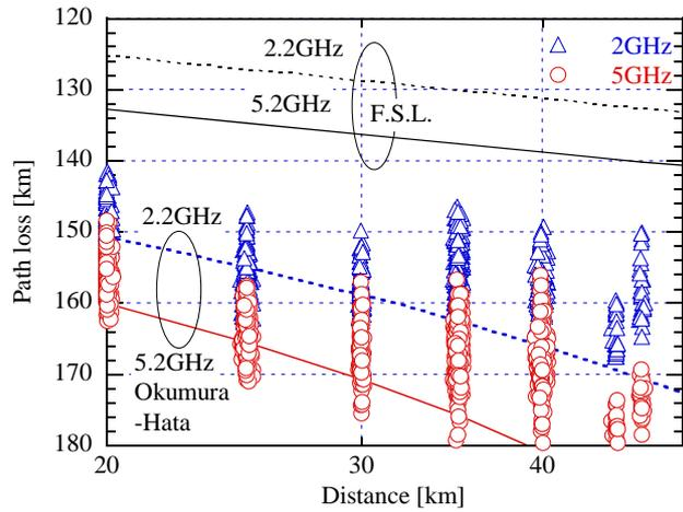
Fig. 9 Path loss vs. distance in Shiroyama-Jujo measurement
