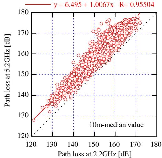
Fig. 5 Path loss correlation between 2.2 GHz and 5.2 GHz in Shinjuku-Kawagoe measurement obtained from 10-m median value
