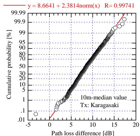
Fig. 14 Path loss correlation between 2.2 GHz and 5.2 GHz in Karagasaki-Chofu measurement obtained from 10-m median value
