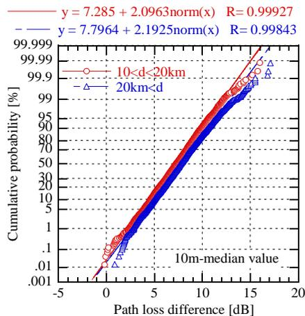
Fig. 7 Cumulative probabilities of the difference in path loss between 2.2 GHz and 5.2 GHz in case of 10-m median value
