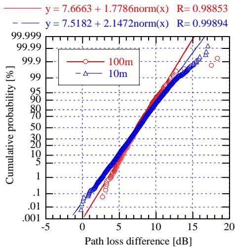
Fig.6 Cumulative probabilities of the difference in path loss between 2.2 GHz and 5.2 GHz
