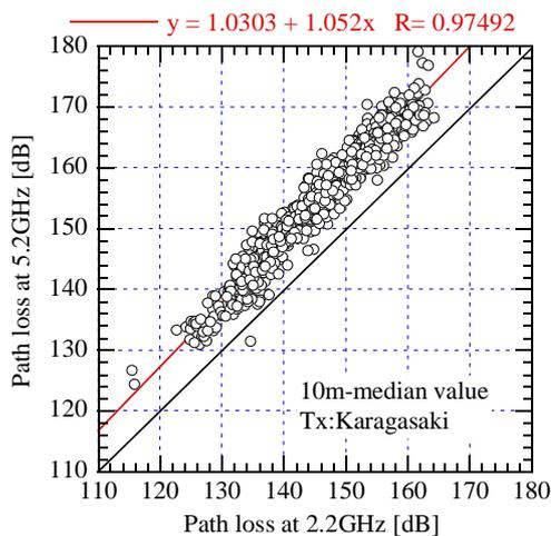
Fig.13 Path loss correlation between 2.2 GHz and 5.2 GHz in Karagasaki-Chofu measurement obtained from 10-m median value
