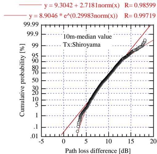
Fig. 11 Cumulative probabilities of the difference in path loss between 2.2 GHz and 5.2 GHz in case of 10-m median value
