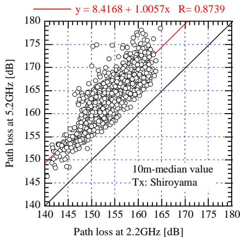
Fig.10 Path loss correlation between 2.2 GHz and 5.2 GHz in Shiroyama-Jujo measurement obtained from 10-m median value
