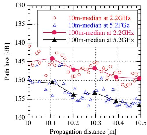
Fig. 3 Example of path loss variations in a short period
